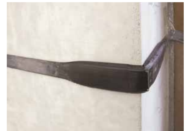
Black Swell before and after swelling with moulded corner
